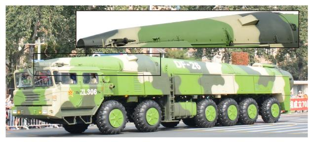
**DF-26 IRBM.** China continues to field the dual-capable DF-26 IRBM that constitutes its first ever precision-strike nuclear capability. The comingling of nuclear and conventional capabilities raises the potential for inadvertent escalation during a conflict. Note the hinged payload access compartment, (inset) which is unique among China's nuclear capable systems. | Image Source: DoD
