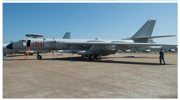
Building Air Based Nuclear Capabilities. The improved H-6N bomber constitutes the nascent air leg of China's nuclear triad. Distinct from the H-6K pictured above and other variants, the H-6N has an air-to-air refueling capability and a recessed fuselage that can carry a nuclear armed air-launched ballistic missile. China intends to surpass this capability with the H-20 stealth strategic bomber that is under development. Image Source: AFP
